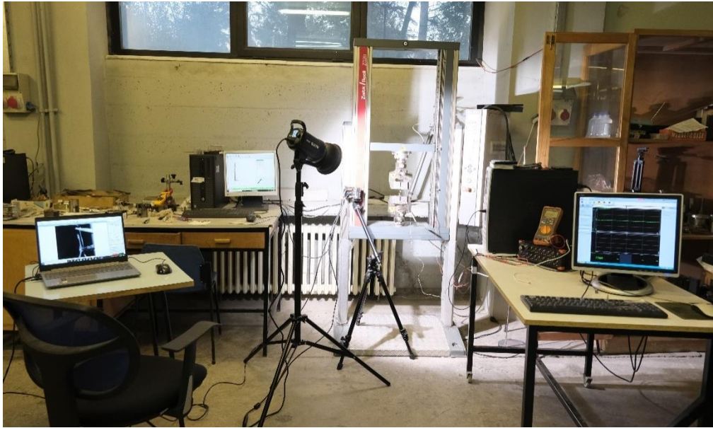
Figure 16. Tensile test and electrical resistance measurements setup.
