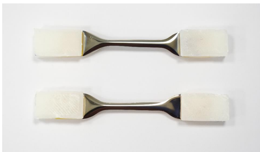
Figure 31. Coated polyimide substrates.
